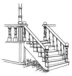
Replacement step railings should match the balustrade of the historic porch in material and detailing:
