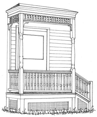
Avoid introducing new materials that were not historically a part of the porch. For example, don't replace wooden posts with brick, metal, or vinyl posts, or with other synthetic material.
